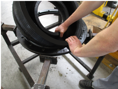
Figure 17: fix bellows to mounting ring
